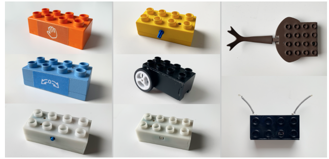
Fig. 4. Sensor bricks (left): tap sensor, incline sensor, button; Actuator bricks (middle): DC motor, wheel, LED; Accessory bricks (right): cephalic horn, bug antennae.
